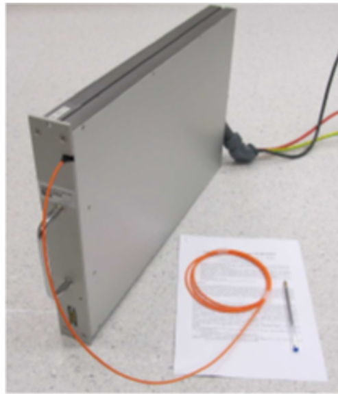
Figure A.2: 1070 nm laser module with approximately 1 kW output ( M^2 \sim 1.1 ; Siewert, 2014)
