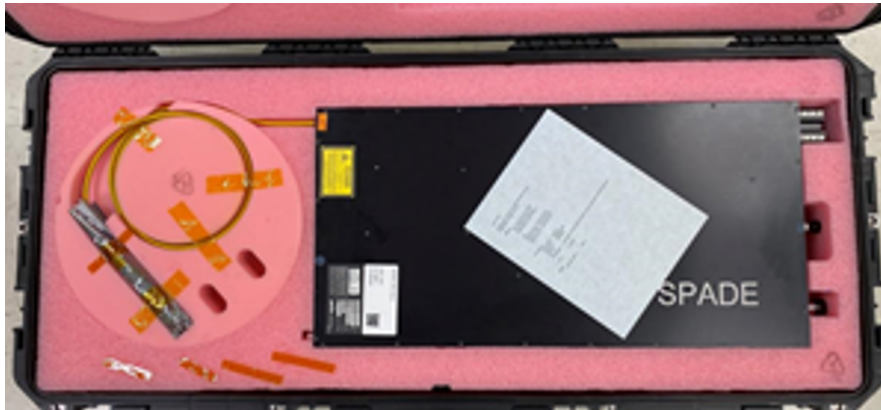
Figure A.3: SPADE amplifier-based laser developed for DSOC Project ground uplink laser assembly.
