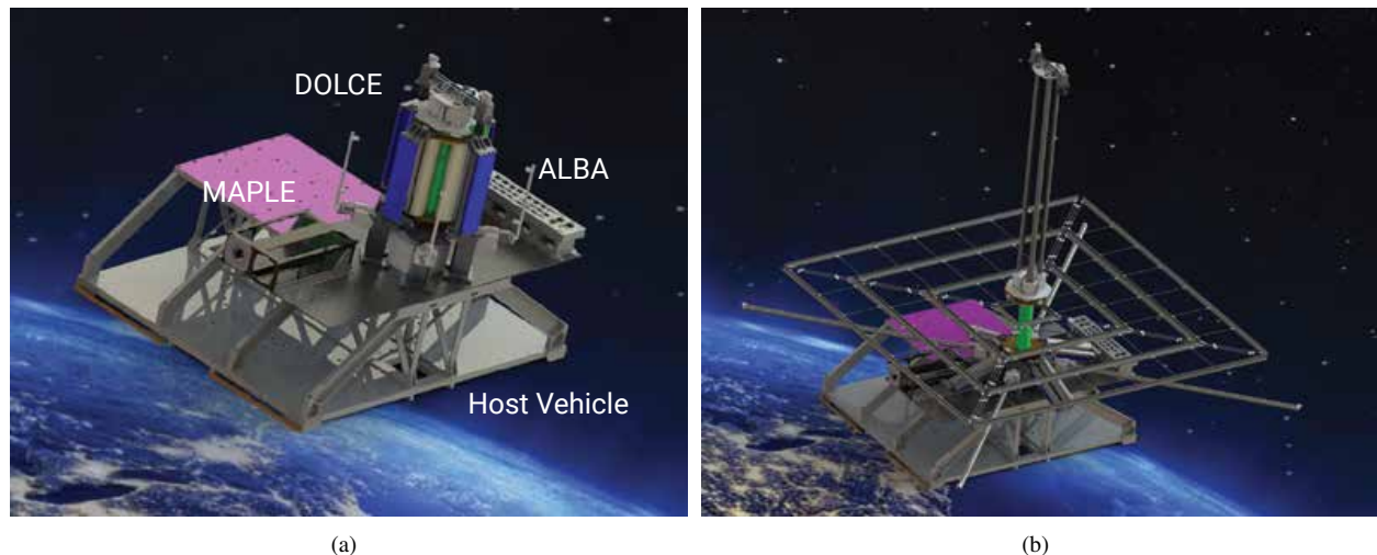
Fig. 1 SSPD-1 rendering on host spacecraft (a) prior to and (b) after DOLCE deployment.
