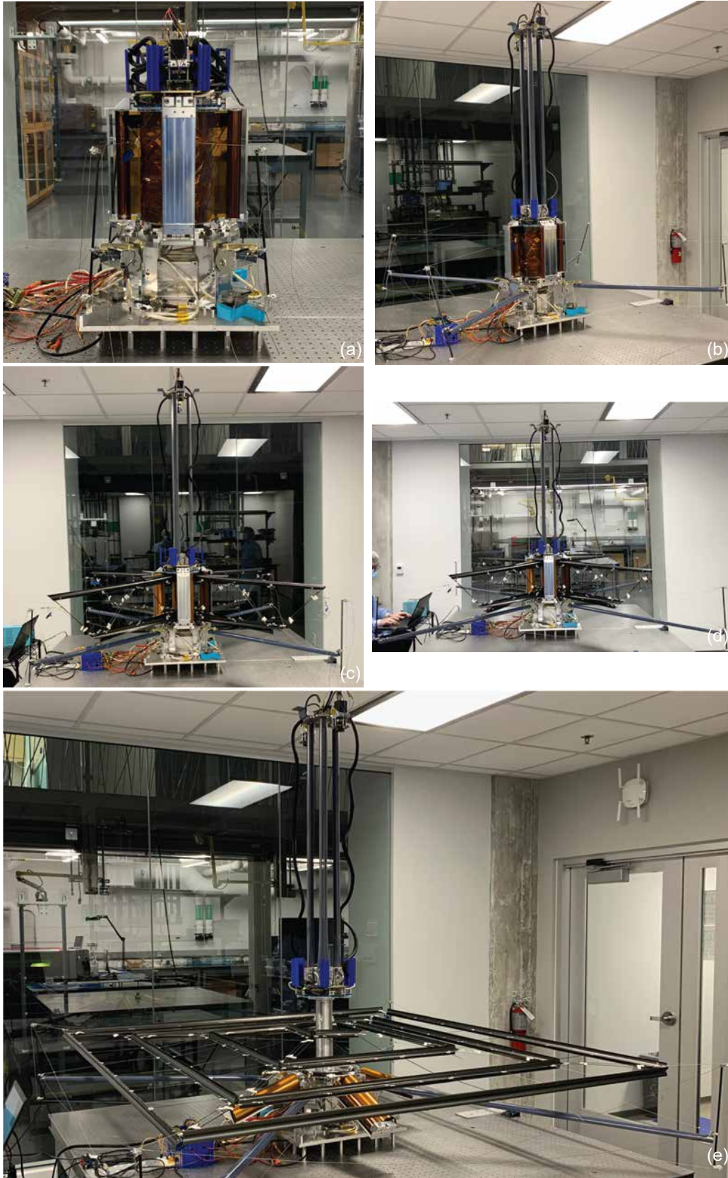
Fig. 13 (a) Integrated DOLCE EM in fully stowed configuration; (b) after complete camera boom deployment and diagonal boom partial deployment; (c) structure uncoiled into the star shape; (d) diagonal boom complete deployment; and (e) after structure complete deployment.
