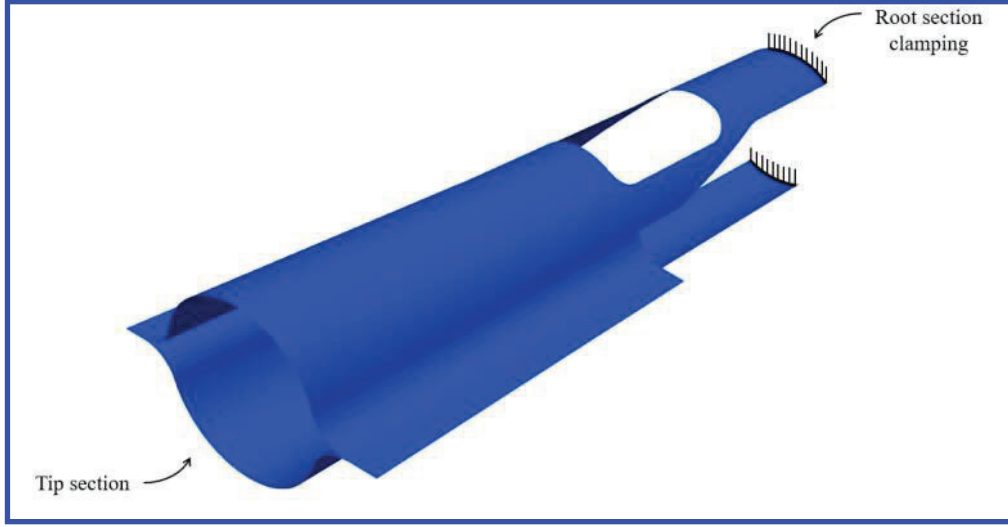
Fig. 2 Partially clamped root cross-section BC concept.
