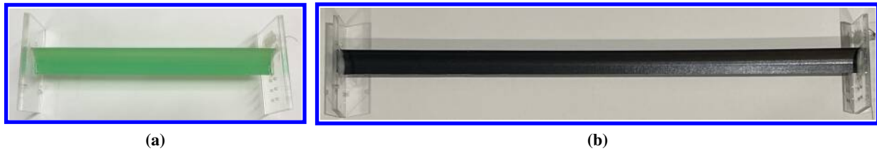
Fig. 4 3D-printed longeron test sample, (a), and composite longeron test sample, (b), glued into acrylic plates.
