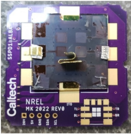
Fig. 4. A sample of a characterization circuit board with a PV device installed.
