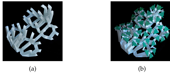
Figure 21: A 3D printed support structure was used to position the prototype in a target surface configuration. (a) Support structure for the T_3 (saddle) configuration. (b) Prototype positioned on the support structure.
