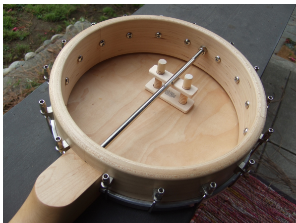
FIG. 7. one of Joel Hooks’ mutes installed to brace the plywood top
