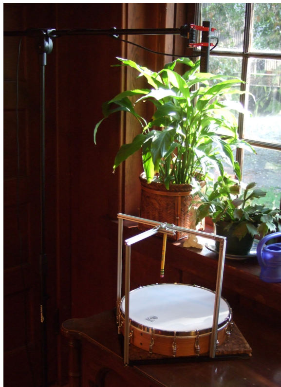
FIG. 3: pencil/pot tap rig and mic
