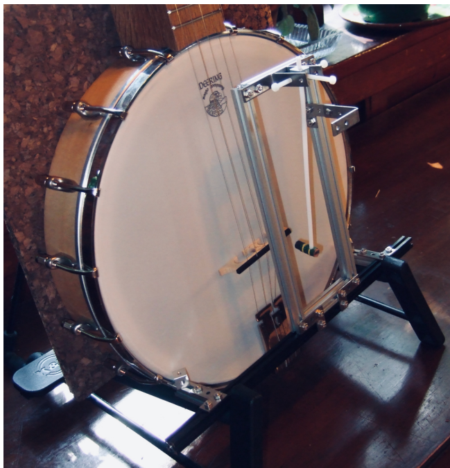
FIG. 9: impulse hammer for bridge taps
