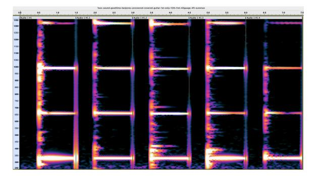
FIG. 11: 1<sup>st</sup> string pluck at 12th fret, tailstrings & all other strings damped, mic at 4'
