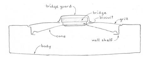
FIG. 3: single-cone (& biscuit) resonator guitar cross section – to scale
