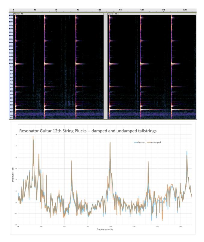
FIG. 9: spectrogram and spectra for plucks on the resonator guitar with cone cover grill and all tailstrings damped on the left and undamped on the right
