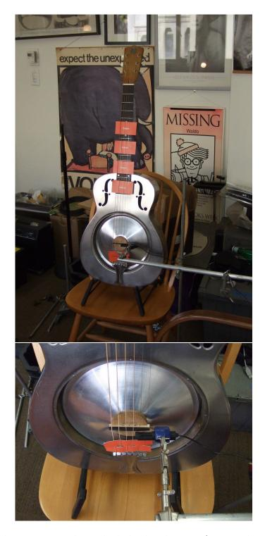
FIG. 4: National resonator with Replogle bridge, biscuit, & cone, damped strings, and mini condenser USB mic, with the protective grill and bridge guard removed
