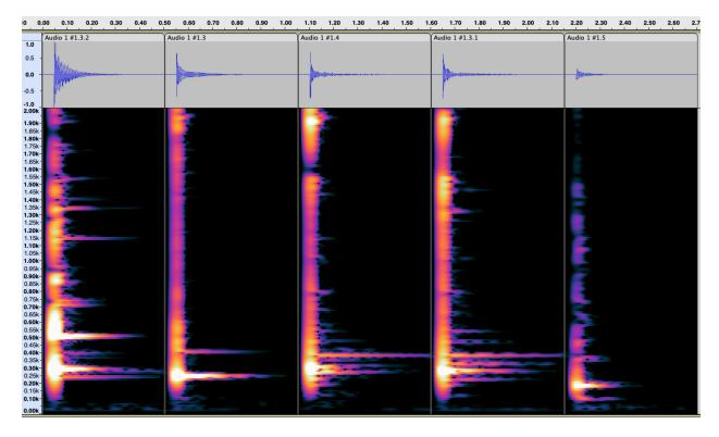
FIG. 5: wave forms and spectrograms of the five damped-string plucks at the bridge
