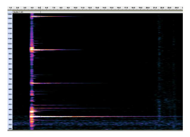
FIG. 13: covered resonator guitar, all open strings, pluck at 12th fret, mic at  $4^\prime$
