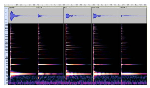
FIG. 10: 1<sup>st</sup> string pluck at 12th fret, tailstrings & all other strings damped, mic at 4'
