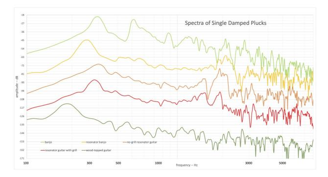
FIG. 7: spectra of the five damped-string plucks at four times lower resolution and successively offset by 20 dB
