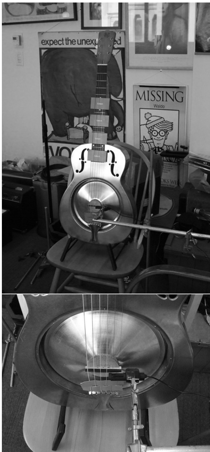
FIG. 4: National resonator with Replogle bridge, biscuit, & cone, damped strings, and mini condenser USB mic, with the protective grill and bridge guard removed
