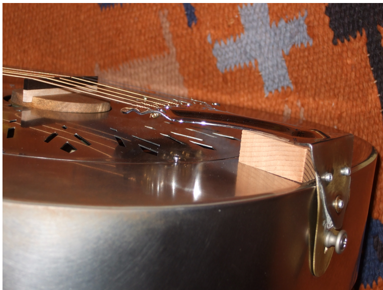
FIG. 3: cover plate installed, bridge and biscuit uncovered, and tailpiece modified to get a 4° break angle with the aluminum & cardstock cones
