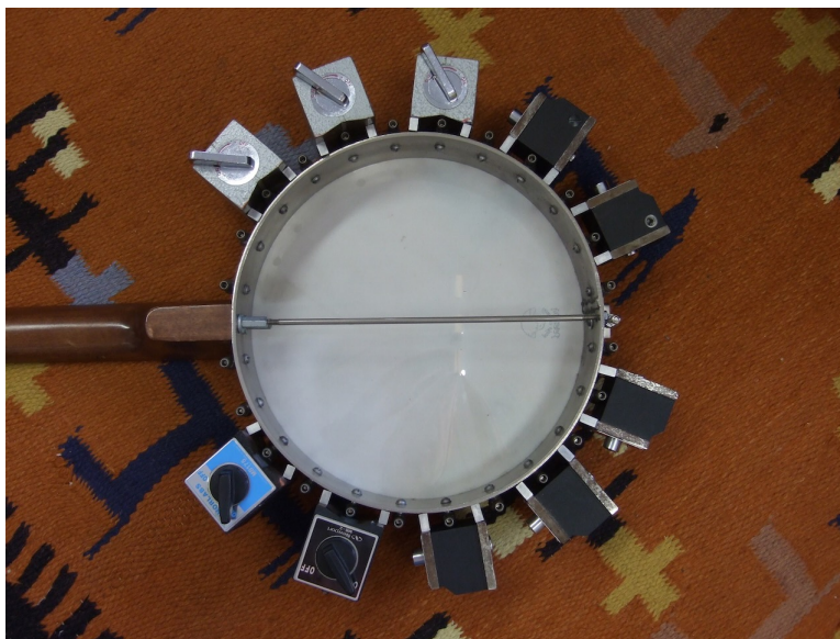
FIG. 11: an extra 14 lbs of magnets attached to the steel rim
