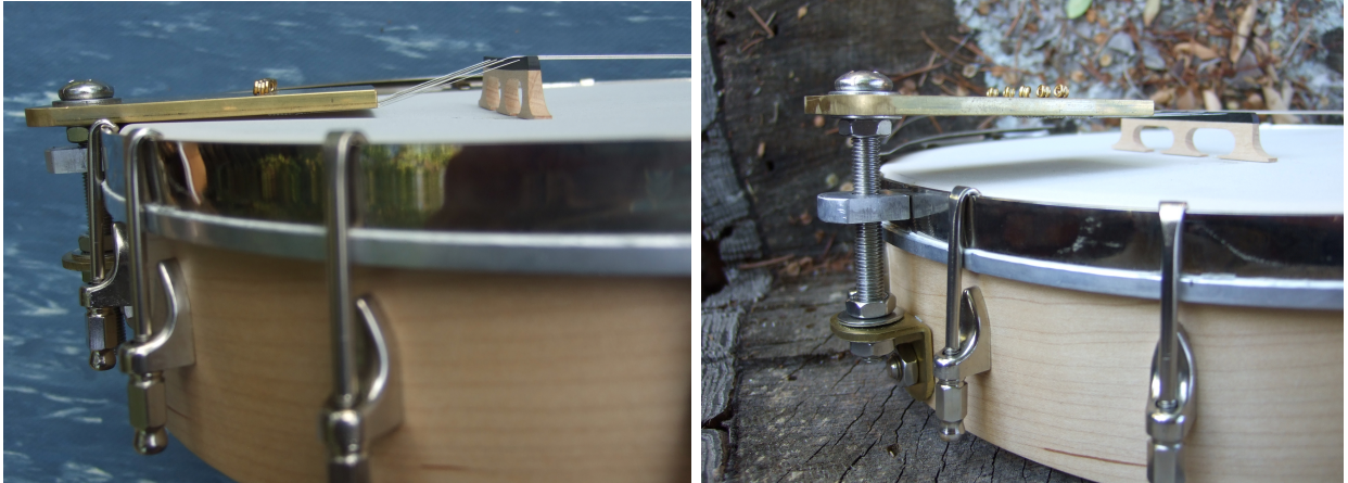
FIG. 1. A simple adjustable tailpiece allows a maximum break angle of 18\frac{1}{2}^\circ (left). The lowest playable angle without a special bridge is 2\frac{1}{2}^\circ (right).
