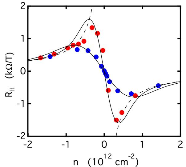
FIG. 3. (Color online) Hall coefficient vs density near the Dirac point. The red and blue data points correspond to  $R_H$  measurements before and after the deposition of about  $2.5 \times 10^{12} \text{ cm}^{-2}$  indium adatoms, respectively. The dashed curve shows the ideal  $R_H = -1/ne$  behavior, while the two solid lines display convolutions of the ideal behavior with Gaussian density distributions of rms width  $\sigma_n = 0.3$  and  $0.6 \times 10^{12} \text{ cm}^{-2}$ .
