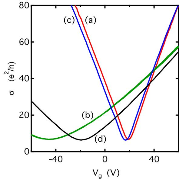
FIG. 2. (Color online) Effect of In deposition on graphene conductivity  $\sigma_{xx}$  vs gate voltage  $V_g$  at  $T = 12 \text{ K}$ . Data is from the wide region of the Hall bar, with trace (a) taken before any In deposition, trace (b) after the first In deposition, trace (c) after warming the sample to  $450 \text{ K}$ , and finally trace (d) after a second In deposition.
