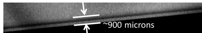
Fig. 3 Resonantly enhanced focused schlieren photo of a laminar boundary layer on a five degree half angle cone in T5, exposure time = 14 microseconds, ( p_{reservoir} = 52 MPa, h_{reservoir} = 8.8 MJ/kg).
