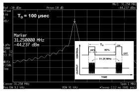
Fig. 8: Typical output spectrum of the transmitter with reference frequency of 1GHz.
