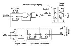
Fig.6: Signal generation circuitry for a single channel of the transmitter.
