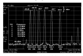
Fig.7: Output spectrum and control signal of Channel-0 in the transmitter.
