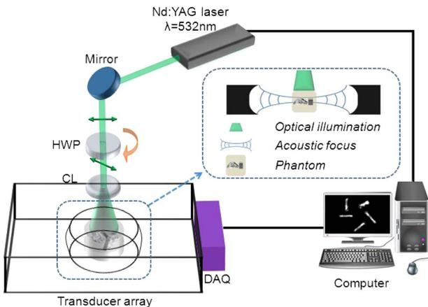
**Fig. 1.** Experimental setup of DS-PACT. The polarization of linearly polarized light is modulated by a half-wave plate, which is driven by a stepper motor. The light is then expanded by a concave lens. HWP, half-wave plate; CL, concave lens; DAQ, data acquisition system.
