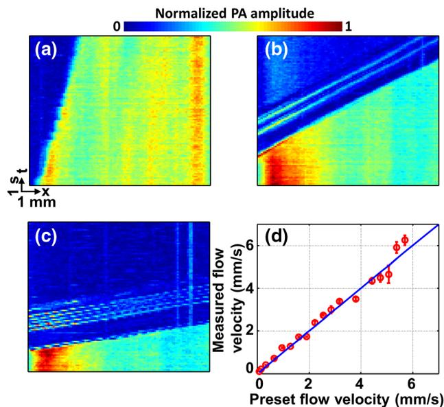
**Fig. 3** Phantom experiments. Time course of the PA amplitude of the blood with flow velocity at (a) 0.2, (b) 1.3, and (c) 4.5 mm/s in a vessel. (d) Measured flow velocity versus preset flow velocity. Red circles, experimental measurement; blue line, ideal fit if the measured and preset velocities are identical.
