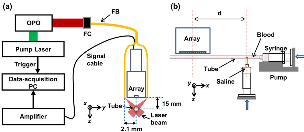
**Fig. 1** Schematic of (a) the photoacoustic tomography system and (b) saline injection. FB, fiber bundle; FC, fiber coupler; OPO, optical parametric oscillator.  $d$  was 15 cm in the phantom experiment.
