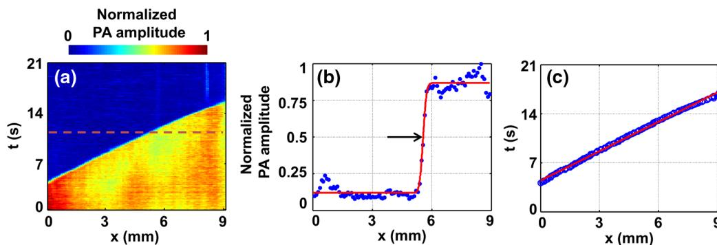
**Fig. 2** Steps to extract the flow velocity. (a) Time course of the photoacoustic (PA) amplitude of the blood vessel in the phantom experiment. (b) Blue dots, one-dimensional PA amplitude along the dashed line in (a); red line, error function fitting; black arrow, the mean value of the error function. The mean value represents the saline–blood interface (SBI). (c) Blue circles, time course of the SBIs; red line, linear fitting.
