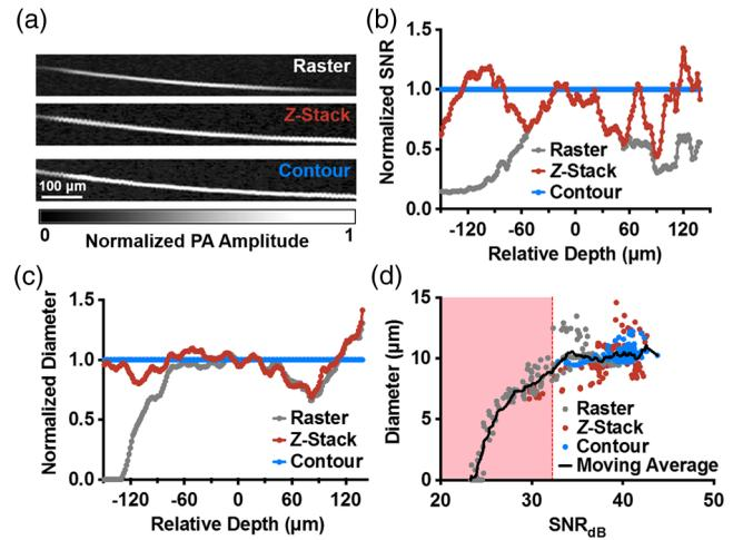
**Fig. 3** Resolution and acoustic-amplitude SNR comparison by imaging a carbon fiber. (a) Top-view maximum amplitude projection (MAP) images of the carbon fiber. (b) Acoustic-amplitude SNR and imaged fiber diameter as a function of fiber depth. (c) Imaged fiber diameter as a function of depth. (d) Diameter as a function of SNR in units of decibels.
