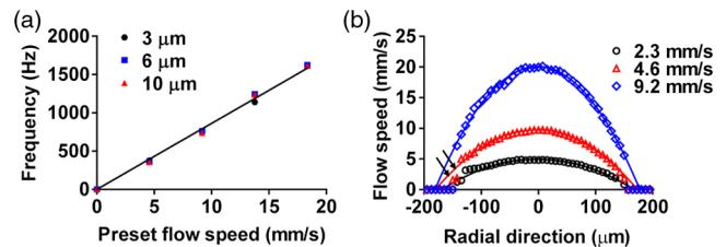
**Fig. 4** Fringe-based PA flowgraphy of microspheres with different diameters. (a) Peak frequency of the PA signal as a function of flow speed with different particle diameters. Solid line: theoretical calculation. (b) Flow speed distribution of 6- $\mu\text{m}$ -diameter particles with different average flow speeds along the radial direction of a cylindrical tube. Solid lines denote parabolic fittings.
