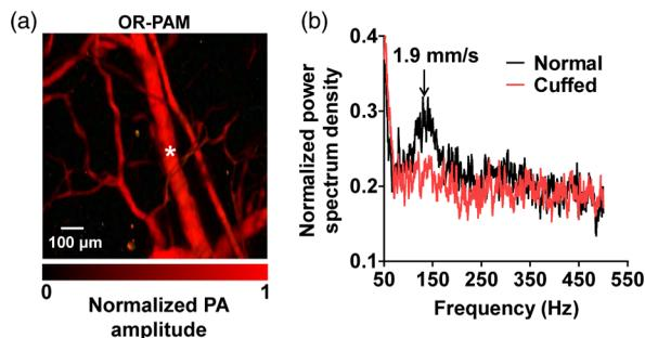
**Fig. 5** Fringe-based PA blood flowgraphy in a mouse ear. (a) Photoacoustic microscopy of the mouse ear vasculature, where the blood flow at the center of a vein was measured, as marked by the star. (b) Frequency spectral densities measured before and after the vein was cuffed.
