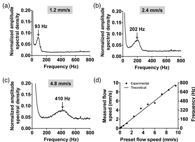
**Fig. 3** Fringe-based PA flowgraphy of whole bovine blood phantom. (a–c) show the normalized amplitude spectral densities for three representative flow speeds. (d) Measured flow speed and peak modulation frequency as a function of the preset speed. The solid line is the theoretical calculation.
