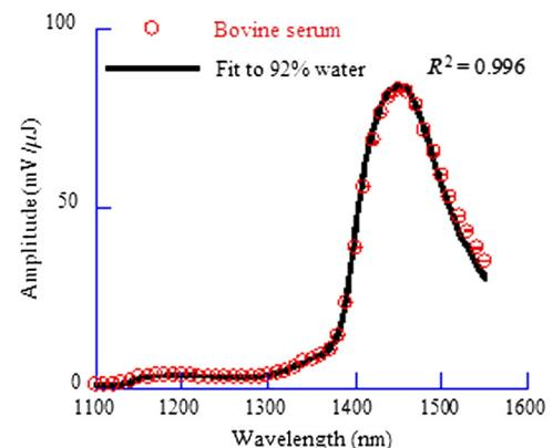
**Fig. 5** Typical photoacoustic spectrum of bovine serum. The normalized amplitude (mean  $\pm$  SE) is plotted versus wavelength. The solid curve is a fit to the absorption spectrum of 92% water, yielding the Grüneisen parameter to be 0.13.
