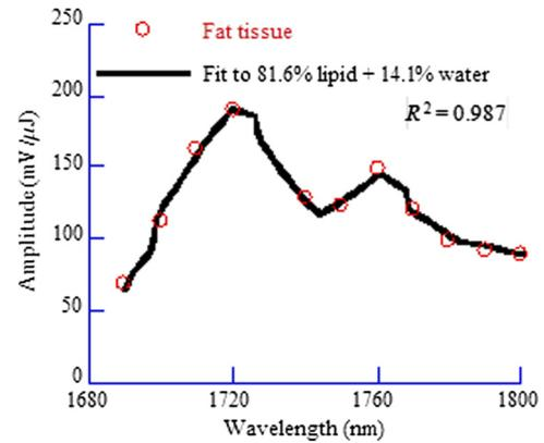
**Fig. 4** Typical photoacoustic spectrum of porcine subcutaneous fat tissue. The normalized amplitude (mean  $\pm$  SE) is plotted versus wavelength. The solid curve is a fit to the absorption spectrum of 81.6% lipid and 14.1% water, yielding a Grüneisen parameter of 0.79.
