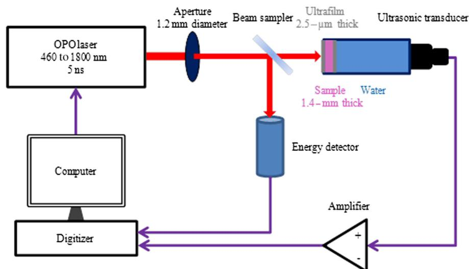
Fig. 1 Schematic of the photoacoustic spectroscopy system.
