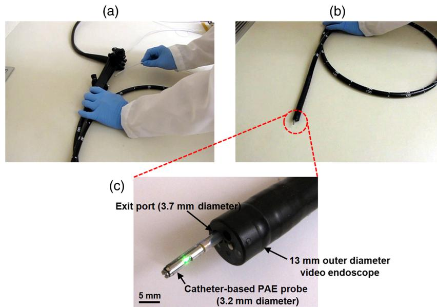
**Fig. 9** Photos of the catheter-based PAE probe positioned fully within (a) and projecting from (b) the 3.7-mm instrument channel of a clinical video endoscope (Video 1, QuickTime, 9.86 MB [URL: <http://dx.doi.org/10.1117/1.JBO.19.6.066001.1>]; Video 2, QuickTime, 3.43 MB) [URL: <http://dx.doi.org/10.1117/1.JBO.19.6.066001.2>]. (c) Magnified view of (b).
