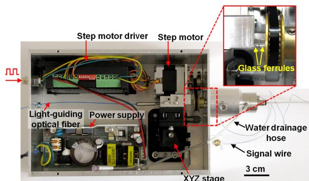
**Fig. 2** Photos of the proximal actuation unit. The inset shows a magnified view of the rotary junction formed for coupling the two multimode optical fibers. The optical fibers are placed inside the two glass ferrules.
