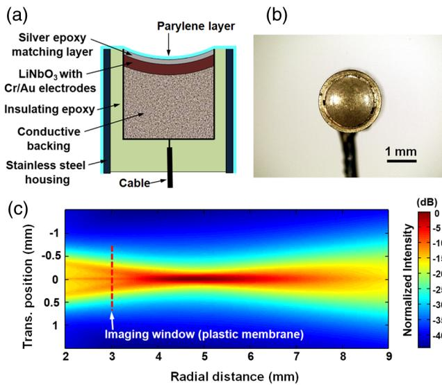
**Fig. 4** Schematic (a) and photo (b) of the focused US transducer implemented by applying the press-focusing technique. (c) Simulated transmission (i.e., one-way) acoustic intensity map of the focused transducer.
