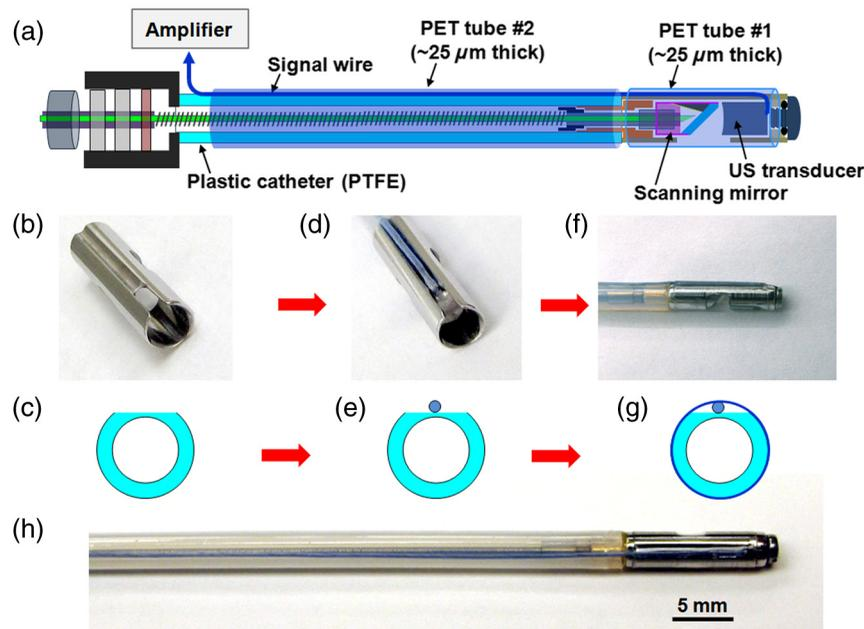
**Fig. 5** (a) Illustration of the affixed US transducer's signal wire. (b–g) Procedure for affixing the signal wire at the stainless steel housing (b, d, f) and plastic catheter (c, e, g). (h) Photo of the catheter probe after affixing the signal wire.
