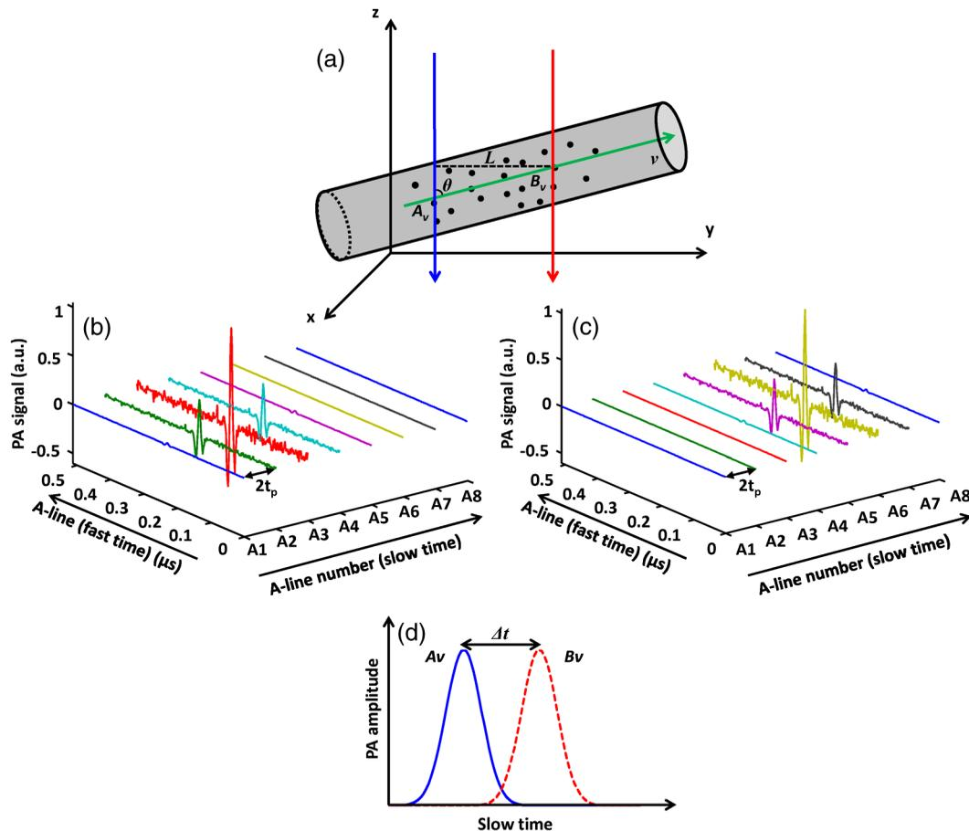
**Fig. 1** Principle of flow measurement by PAM based on cross correlation. (a) Two laser beams (blue and red arrows) illuminate the measurement area of a blood vessel alternately. The axes of the two beams are separated by distance  $L$ . Sequential A-lines are acquired at (b)  $A_v$  and (c)  $B_v$  at an interval time of  $2t_p$ . (d) The slow-time photoacoustic (PA) profiles from  $A_v$  and  $B_v$  are shifted in time by  $\Delta t$ .
