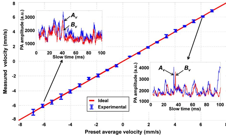
**Fig. 3** Measured transverse flow velocities using 10- $\mu\text{m}$ -diameter microspheres. Inset figures show raw slow-time PA profiles from  $A_v$  (blue) and  $B_v$  (red) in Fig. 1 at two selected flow velocities  $v = +6.14 \text{ mm/s}$  and  $v = -6.14 \text{ mm/s}$ . Error bars: standard errors.
