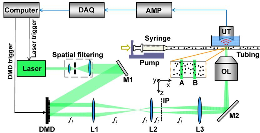
**Fig. 2** Schematic overview of the setup, not to scale. AMP, signal amplifiers and filters; DAQ, data acquisition; DMD, digital micromirror device; IP, intermediate image plane; L1–L3, lenses (focal lengths  $f_1 - f_3$ ); M1 and M2, mirrors; OL, objective lens; UT, ultrasound transducer.
