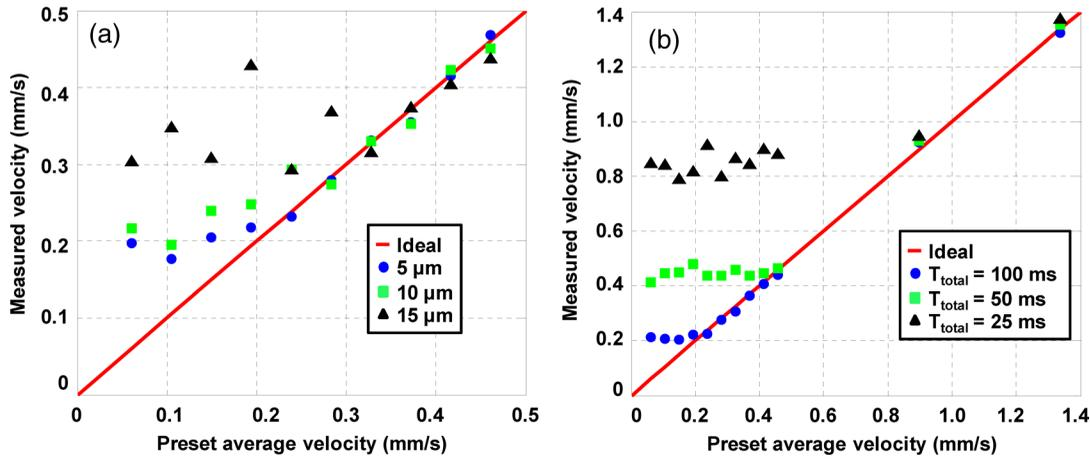
**Fig. 7** Quantification of the minimum measurable flow velocity  $|v_{\min}|$  for 10- $\mu\text{m}$ -diameter microspheres. (a) Measured flow velocities for three different distances at slow preset flow velocity range  $|v| = 0.06\text{--}0.46$  mm/s for a fixed time  $t_{\text{total}} = 100$  ms. (b) Measured flow velocities using three different  $t_{\text{total}}$  at a fixed distance  $L = 5$   $\mu\text{m}$ .
