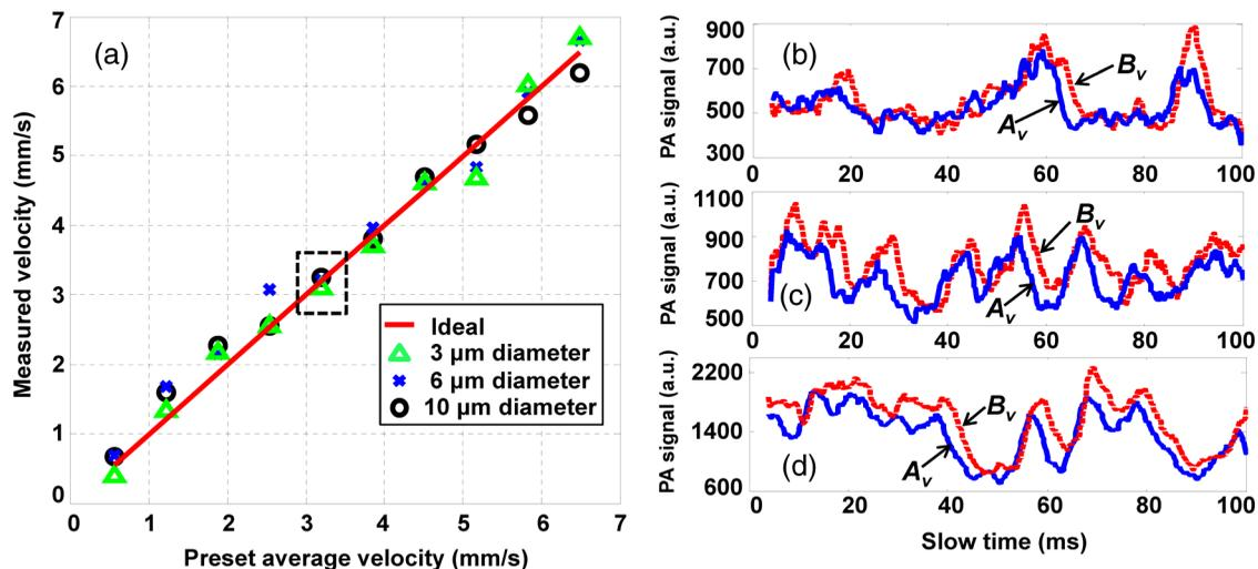
**Fig. 4** (a) Flow velocities measured using three sizes of microspheres. (b)–(d) The slow-time PA profiles from  $A_v$  (blue solid line) and  $B_v$  (red dashed line) in Fig. 1 with the same flow speed [dashed box in (a)] for (b) 3  $\mu\text{m}$ , (c) 6  $\mu\text{m}$ , and (d) 10- $\mu\text{m}$ -diameter microspheres. The calculated average time shift between the blue and red slow-time PA profiles is the same regardless of individual profile shapes.
