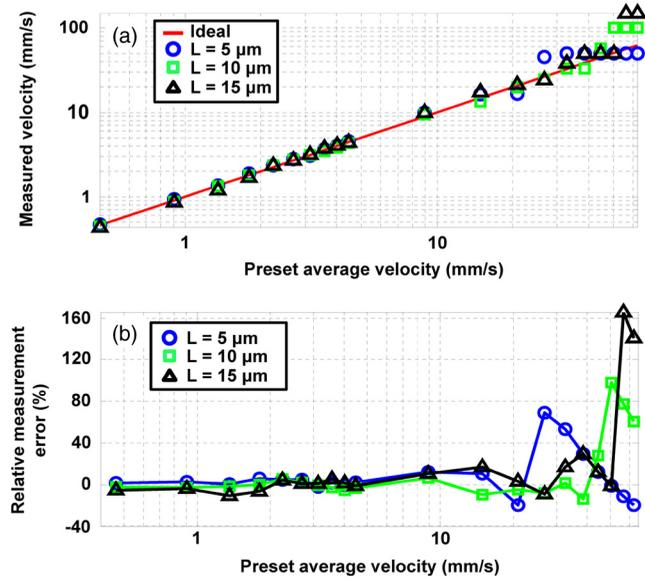
Fig. 6 Quantification of the maximum measurable velocities for 10- $\mu\text{m}$ -diameter microspheres. (a) Log-log plot of the measured flow velocities for three different distances. (b) Semi-log plot of the relative errors of the measured velocities.
