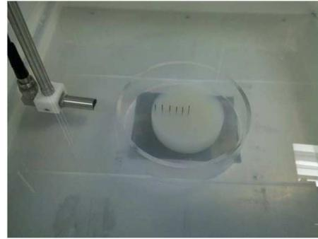
Fig. 3. Photograph of the pencil leads held in agar and surrounded by an acrylic cylindrical shell.
