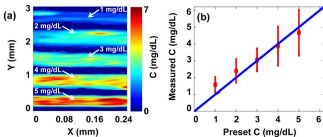
**Fig. 4** Quantitative PAM of tissue-mimicking samples containing bilirubin with varied concentrations. (a) Bilirubin distribution image. From top to bottom in the image, the sample concentrations are 1, 2, 3, 4, and 5 mg/dL, respectively. (b) Volume-averaged bilirubin concentrations from the PAM measurements in each sample. Red circle: experimental measurement. Blue line: ideal fit if the measured and preset concentrations are identical.
