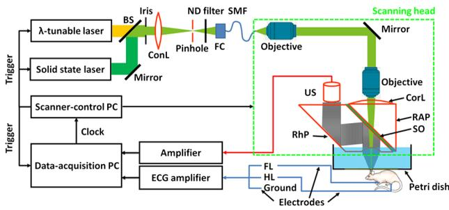
**Fig. 1** Schematic of the ECG-synchronized OR-PAM system for PWV measurement.  $\lambda$ , wavelength; BS, beam splitter; ConL, condenser lens; ND, neutral density; FC, fiber collimator; SMF, single-mode fiber; CorL, correction lens; RAP, right-angle prism; SO, silicone oil; RhP, rhomboid prism; US, ultrasonic transducer; FL, foreleg; HL, hind leg; PC, personal computer.
