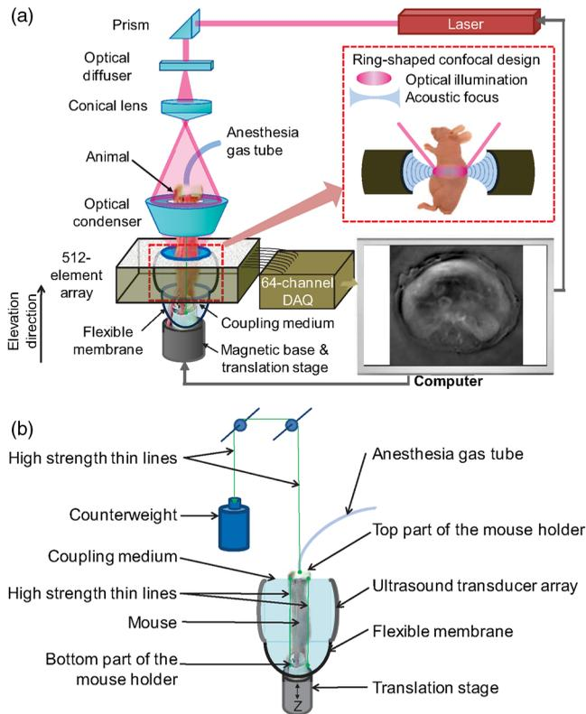
**Fig. 1** Experimental setup of the full-ring confocal whole-body photoacoustic computed tomography (RC-PACT) system. (a) Schematic of the RC-PACT system. The dashed box shows a cross-sectional view of the confocal design. (b) A detailed view of the animal holder.
