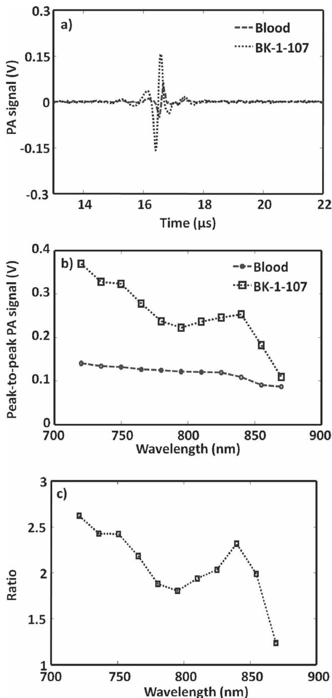
**Figure 2.** PA imaging of NIR polymer nanoparticle against blood. a) PA spectroscopy signals generated from a tygon tube (I. D. 250  $\mu\text{m}$ , O. D. 500  $\mu\text{m}$ ) filled with NIR-polymer micelle and rat blood. The laser was tuned to 750 nm wavelength. b) PA spectrum of NIR-polymer micelle and rat blood over a 720–870 nm NIR wavelength range. c) Ratio of the peak-to-peak PA signal amplitudes generated from polymeric nanoparticle to those of blood.
