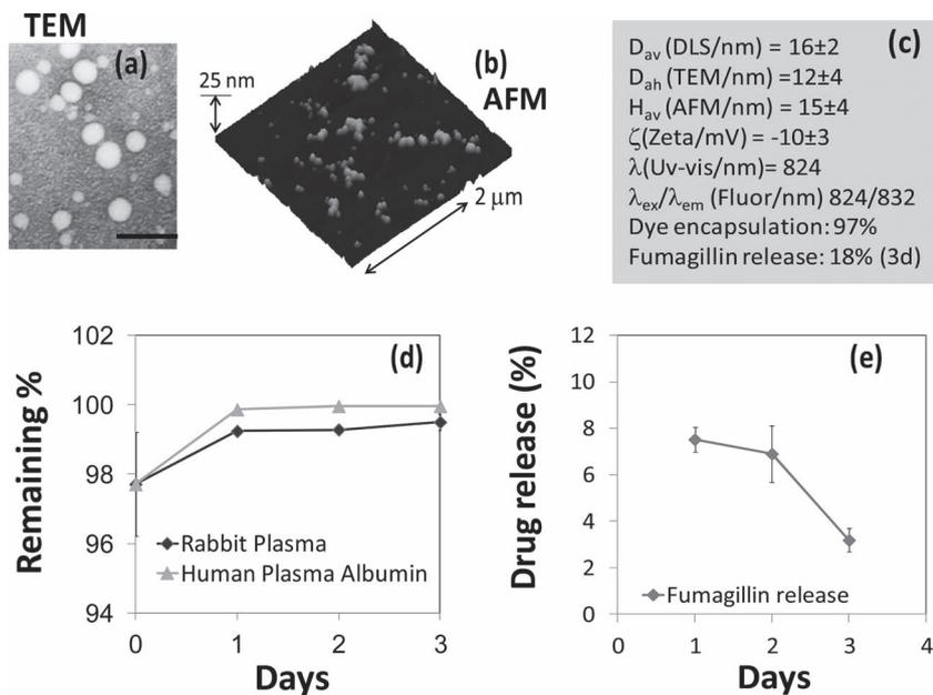
**Figure 1.** a) TEM image of the polymeric micelles drop deposited over nickel grid, scale bar = 100 nm; b) AFM image of the micelles drop deposited over glass; c) physico-chemical characterization table for a NIR-polymer micelle; d) dissolution of ADS-832-WS from micelle when incubated against rabbit plasma and human plasma albumin; (e) time-dependent release of fumagillin from micelle.
