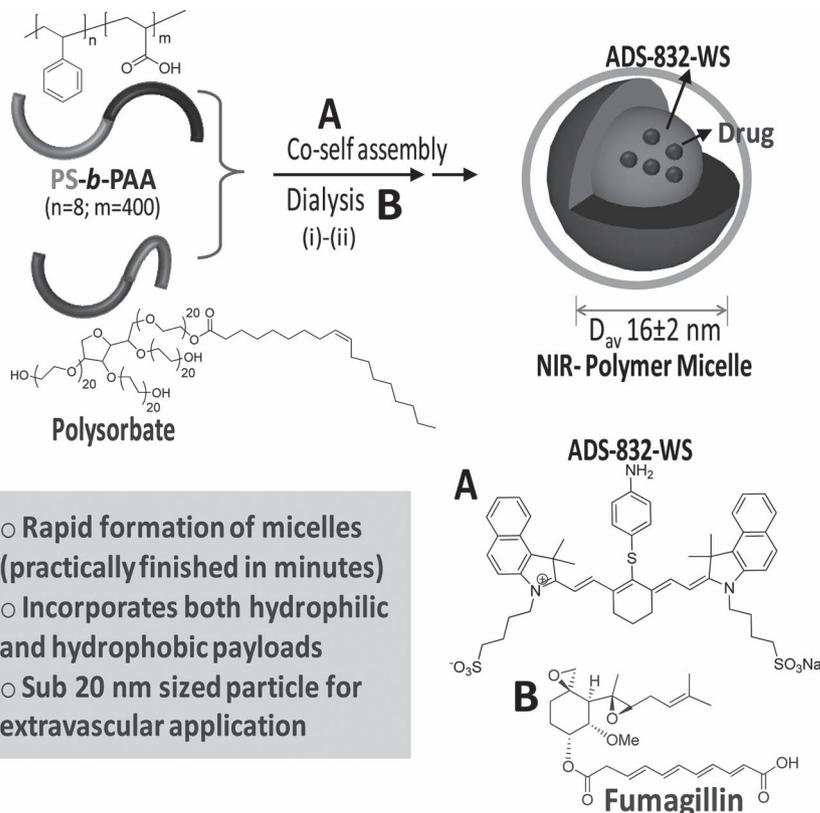
**Scheme 1.** Synthesis and characterization of theranostic polymeric micelles: i) co-self assembly of amphiphilic diblock copolymer and sorbitan monooleate, ADS-832-WS (A) and/or fumagillin (B), sonication, 25 °C, 1 min; ii) dialysis 10 kDa cellulose membrane, nanopure water (0.2  $\mu\text{M}$ ).
