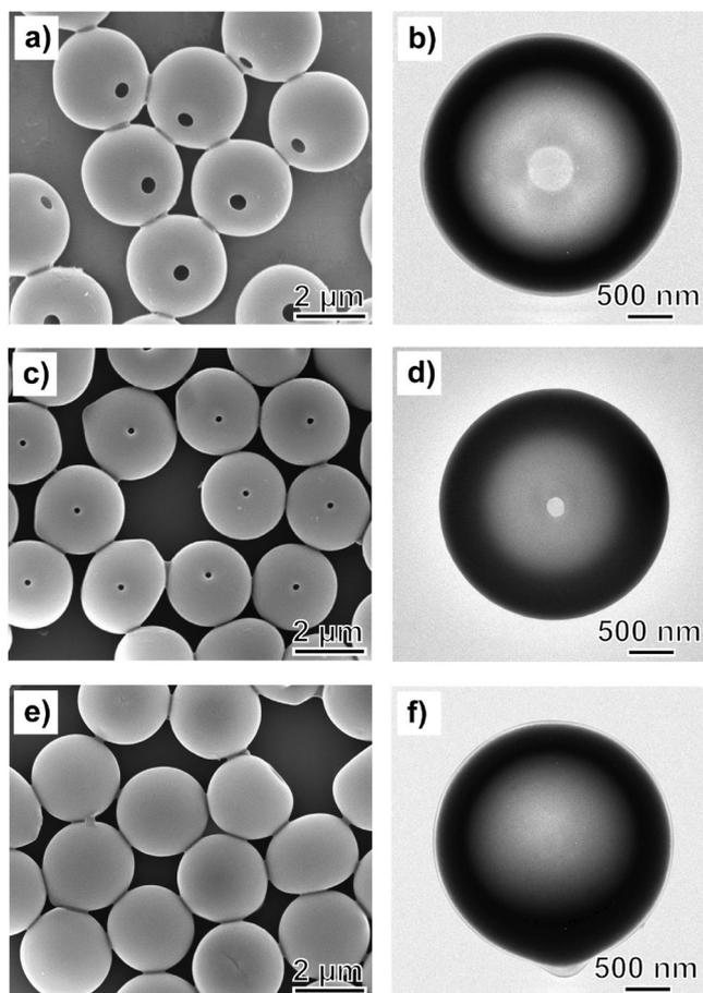
**Figure 2.** a) SEM and b) TEM images of the as-prepared PS hollow beads with holes on their surfaces. c) SEM and d) TEM images of the same batch of PS hollow beads where the holes had been partially closed by annealing the system in water at 95 °C for 5 min. e) SEM and f) TEM images of the same batch of PS hollow beads where the holes had been completely closed by annealing the system in water at 95 °C for 30 min.
