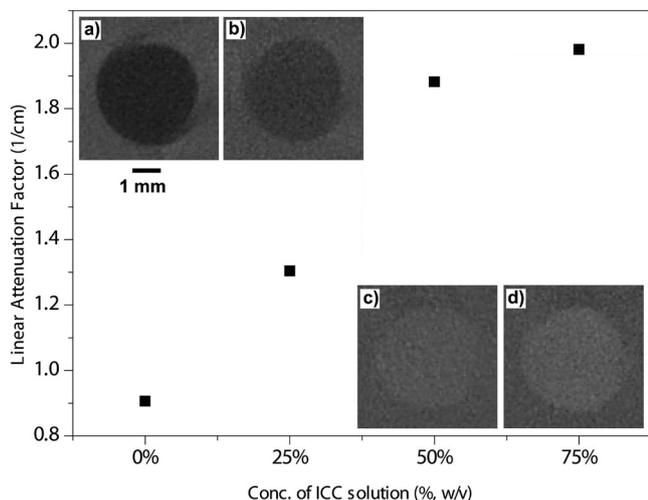
**Figure 7.** microCT imaging of PS hollow beads containing aqueous ICC solutions with different concentrations (used for encapsulation): a) 0%, b) 25%, c) 51%, and d) 74%. The squares shown in the figure indicate the average values of linear attenuation factors for each accompanying microCT image. The 1 mm scalebar is the same for all microCT images.
