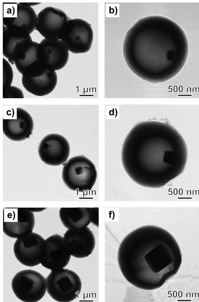
**Figure 3.** TEM images of the PS hollow beads that had been encapsulated with saline solutions of different concentrations: a,b) 5.9 wt%, c,d) 11.1 wt%, and e,f) 23.1 wt%. The holes were closed by annealing the samples in the corresponding saline solutions at 95 °C for 45 min. The samples were collected by centrifugation and thoroughly washed with water. The samples supported on copper grids were further dried at 75 °C for 5 min to completely remove water prior to TEM characterization.
