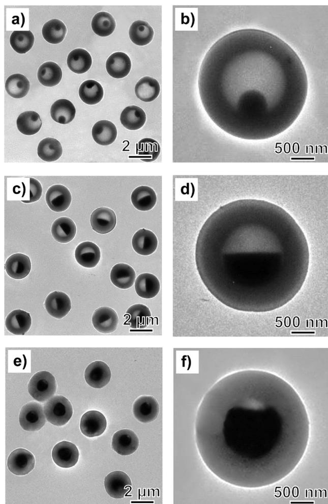
**Figure 4.** TEM images of PS hollow beads containing ioversol in the interiors. The holes were closed by heating the PS hollow beads at 95 °C for 45 min in aqueous solutions containing: a,b) 25%, c,d) 51%, and e,f) 74% of ioversol. The samples were collected by centrifugation and thoroughly washed with ethanol and dried at 75 °C for 5 min to completely remove the water inside the beads prior to TEM characterization.
