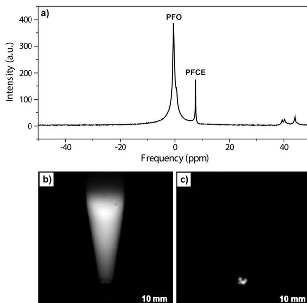
**Figure 5.** MR spectrum and images of PS hollow beads whose interiors had been encapsulated with PFO: a) a  $^{19}\text{F}$  MR spectrum acquired from a sample containing PFO-encapsulated PS hollow beads and perfluoro-15-crown-5-ether (PFCE), a reference compound; b)  $^1\text{H}$  mapping image from a suspension containing PFO-encapsulated PS hollow beads hosted in a centrifuge tube; and c)  $^{19}\text{F}$  mapping image of the same sample by using the peak of PFO.
