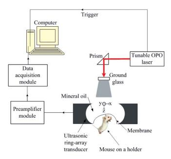
Fig. 1 Schematic of the photoacoustic tomography system.
