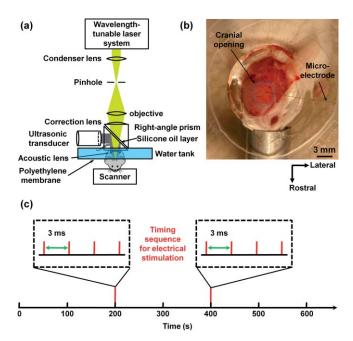
**Fig. 1** (a) Schematic of the optical-resolution photoacoustic microscope. (b) Photograph of the exposed mouse brain surface with an introduced microelectrode. (c) Timing sequence for electrical stimulation.
