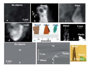
**Fig. 2** PA images and digital photographs for various foreign bodies. Objects were embedded in chicken breast tissue: (a) PA MAP image without objects embedded in the tissue, (b–d,f) PA MAP images, (e,i) digital photographs, (g) PA B-scan image without objects embedded in the tissue, and (h) PA B-scan images. TS: tissue surface.
