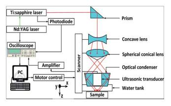
Fig. 1 Schematic of the deep-penetrating reflection-mode photoacoustic imaging system. A Cartesian coordinate is shown.
