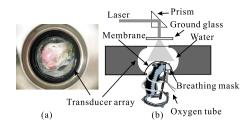
**Fig. 1** Full-ring array PAT system. (a) Top view of the full-ring array and the animal head. (b) Side view of the array system and the position of the animal.
