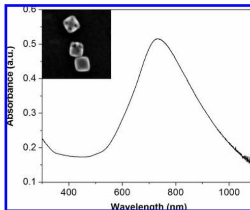
**Figure 1.** Absorption spectrum of Au nanocages. Wavelength at peak optical absorption was  $\sim 735$  nm. Inset shows a typical SEM image of the Au nanocages with the scale bar being 50 nm. The average edge length was  $50.3 \pm 6.7$  nm (standard deviation). The Au nanocages were stabilized with polyvinyl pyrrolidone (PVP).
