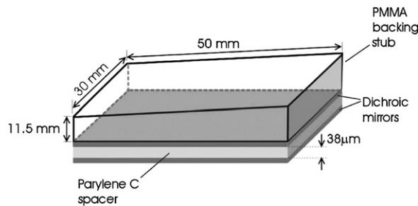
**Figure 3.** Schematic of an FP sensor head. The sensing structure comprises a  $38\ \mu\text{m}$  polymer (Parylene C) film spacer sandwiched between two dichroic mirrors, forming an FPI. The latter overlays a PMMA backing stub that is wedged to eliminate parasitic interference between light reflected from its upper surface and the FPI. Reprinted with permission from Zhang *et al* (2008).
