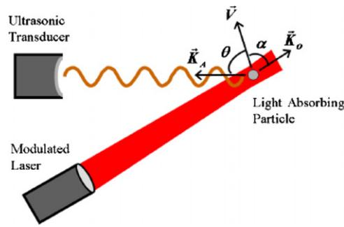
**Figure 13.** Schematic for the photoacoustic Doppler shift. The small light-absorbing particle moving along the velocity vector is illuminated by modulated continuous-wave light.  $\vec{K}_0$ ,  $\vec{V}$  and  $\vec{K}_A$  represent the directions of laser illumination, velocity of the absorber and acoustic waves, respectively. Reprinted with permission from Fang *et al* (2007). Copyright (2007) by the American Physical Society.
