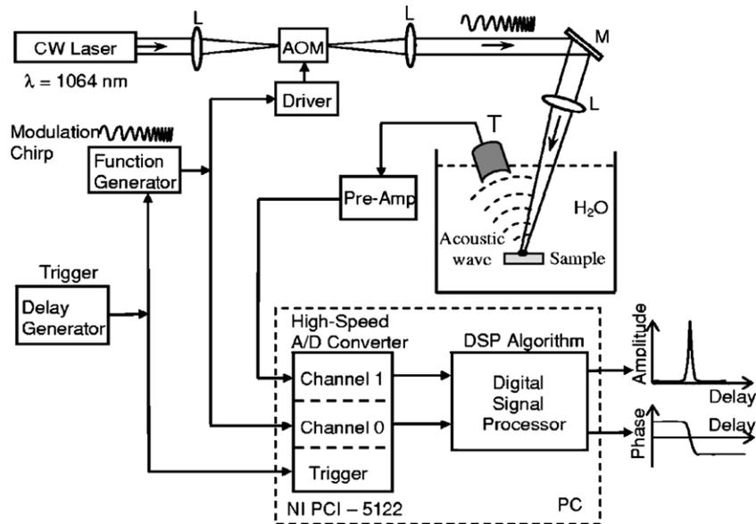
**Figure 7.** Schematic diagram of the frequency-domain PA imaging system with a frequency-swept laser source. AOM-acousto-optic modulator, L-lenses, M-mirror, T-ultrasonic transducer. Reprinted with permission from Telenkov and Mandelis (2006).
