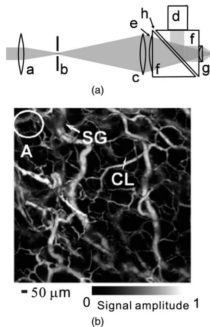
**Figure 6.** (a) Schematic of the OR-PAM system. a, condenser lens; b, pinhole; c, microscope objective; d, ultrasonic transducer; e, correcting lens; f, isosceles prism; g, acoustic lens; h, silicon oil. (b) *In vivo* OR-PAM image of microvasculature in a nude mouse ear. CL, capillary, and SG, sebaceous gland. Reprinted with permission from Maslov *et al* (2008).
