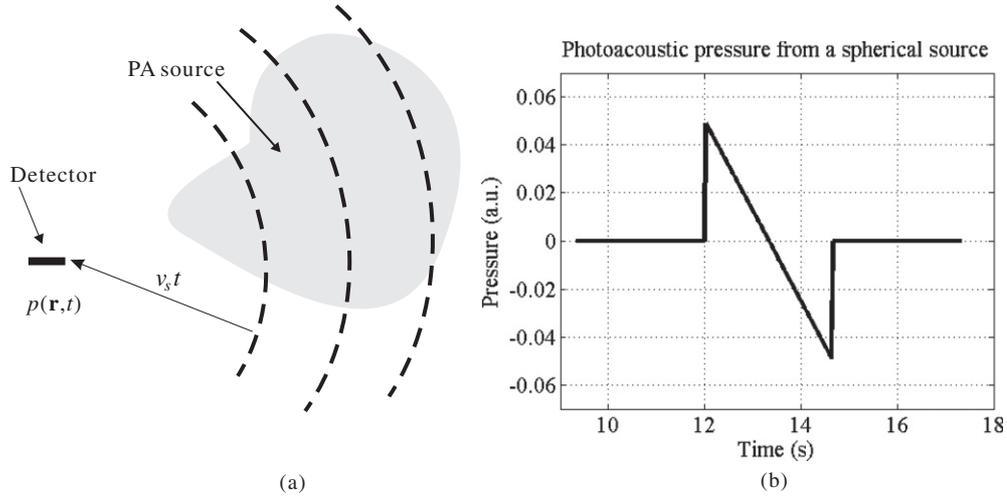
**Figure 2.** (a) The PA waves detected by a point detector at a certain time  $t$  come from sources over a spherical shell centered at the detector position and a radius of  $v_s t$ . (b) An example of the pressure generated by a uniform spherical PA source.
