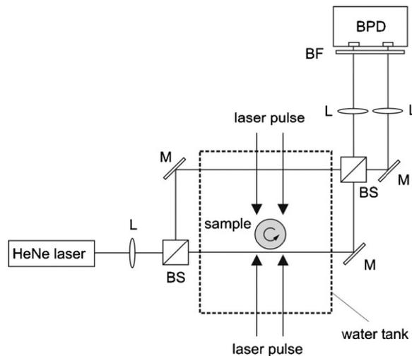
**Figure 4.** Experimental setup for photoacoustic tomography with a Mach–Zehnder interferometer as acoustic line detector. BS, beam splitter; M, mirror; BPD, balanced photodetector; L, lens; BF, bandpass filter. Reprinted with permission from Paltauf *et al* (2007).
