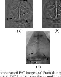
**Fig. 3** Reconstructed PAT images. (a) From data gathered by a positively focused PVDF transducer; the scanning radius of the virtual point was 2.7 cm. (b) From data gathered by a flat transducer; the scanning radius was 4.1 cm. (c) Photograph of the mouse cortex taken after photoacoustic data acquisition.
