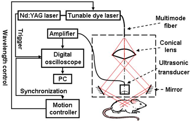
Fig. 1. Schematic of the dual-wavelength photoacoustic microscopy system.
