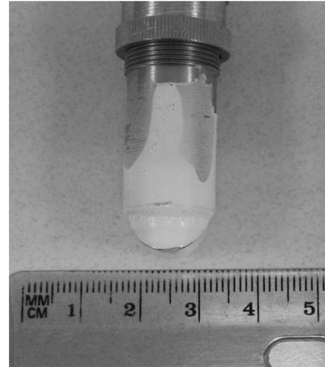
FIG. 4. A negative cylindrical lens made from acrylic plastic is epoxied to the surface of an ultrasound transducer. The lens and part of the transducer are painted white with silica gel to diminish the absorption of laser light illuminating on the transducer.
