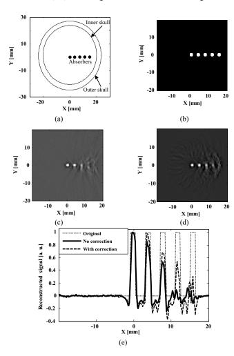
Fig. 3. Numerical simulation: (a) Schematic illustration of the phantom sample used in the simulation; (b) close-up view of the five absorbers, shown as white spots in the imaging area; (c) reconstructed TAT image without correction for skull effects; (d) reconstructed image after correction for skull effects; and (e) comparison of the reconstructed signals across the five absorbers.
