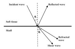
Fig. 1. Schematic illustration of the reflection, refraction, and mode conversion of longitudinal incident waves.
