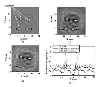
Fig. 6. Reconstructed TAT image: (a) Using the filtered back-projection method when skull was absent; (b) using the filtered back-projection method when skull was present; (c) using the proposed numerical method when skull was present; (d) comparison of the reconstructed signals at the depth as marked on (a), (b), and (c). We shifted the positions of the plots for (b) and (c) along the y axis by -0.3 and -0.7, respectively.
