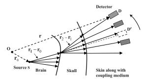
Fig. 2. Schematic illustration of forward TAT propagation.
