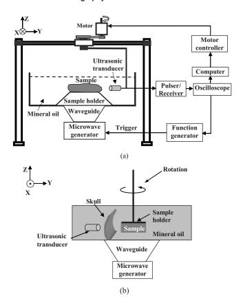
Fig. 4. (a) Schematic of the experimental setup and (b) side view of experimental setup using a piece of monkey skull bone.
