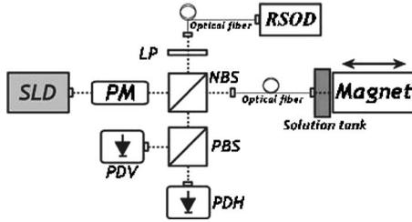
**Fig. 2** Schematic of the PS-OCT setup. SLD—superluminescent diode; PM—polarization modulator; NBS—nonpolarizing beamsplitter; PBS—polarizing beamsplitter; LP—linear polarizer; RSOD—rapid scanning optical delay line; PDH—horizontal detector; PDV—vertical detector.
