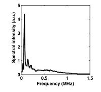
Fig. 2. Average temporal spectral intensity of the thermoacoustic signals corresponding to Fig. 3.
