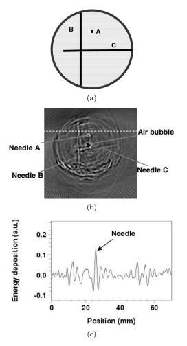
Fig. 4. (a) Diagram showing a monkey head with three inserted needles. (b) TAT image. (c) The line plot along the dashed line in (b).
