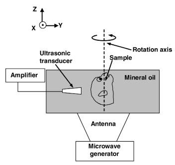
Fig. 1. Diagram of the experimental setup.
