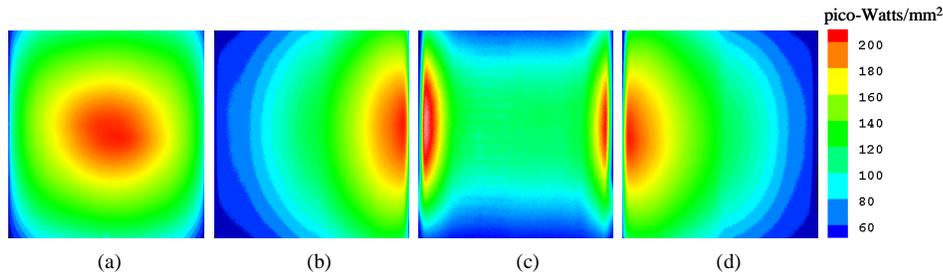
Fig. 12. Luminescent views of the side surface covering cylindrical phantom taken using a CCD camera in four directions 90 degrees apart. (a) Front view, (b) Right view, (c) Back view, and (d) Left view.
