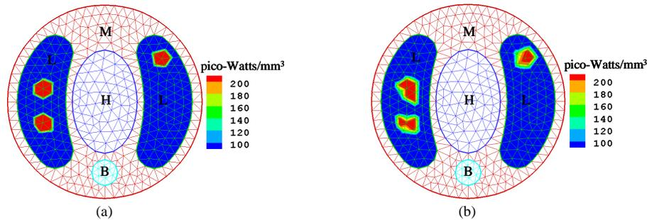
Fig. 4. Numerical simulation for BLT reconstruction of three sources: two in the left lung and one in the right lung. (a) The true source distribution in which each source consists of several volume elements and has density 200.0 pW/mm<sup>3</sup>, and (b) the counterparts reconstructed from the surface data corrupted by 10% Gaussian noise. The average density error is 3%.
