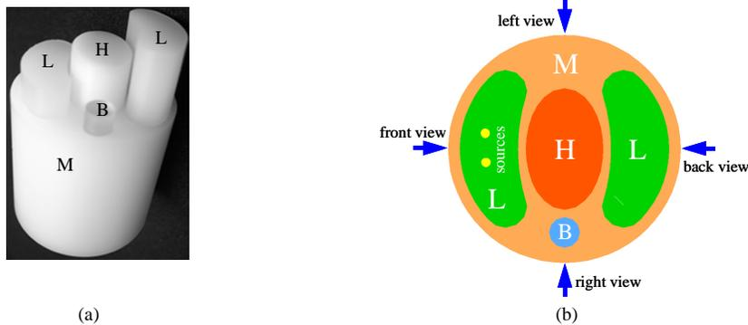
Fig. 10. Mouse Chest phantom. (a) A heterogeneous mouse phantom consisting of bone (B), heart (H), lungs (L), and muscle (M); (b) a middle cross-section through two hollow cylinders for hosting luminescent sources in the left lung. The four arrows show the direction of the CCD camera during data acquisition.
