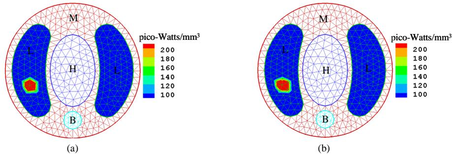
Fig. 1. Numerical simulation for BLT reconstruction of one source. (a) The true source distribution in the left lung consisting of 6 volume elements and having a homogeneous density of  $200.0\text{pico-Watts/mm}^3$ , and (b) the counterpart reconstructed from the surface data corrupted by 10% Gaussian noise. The average density error is 0.5%.
