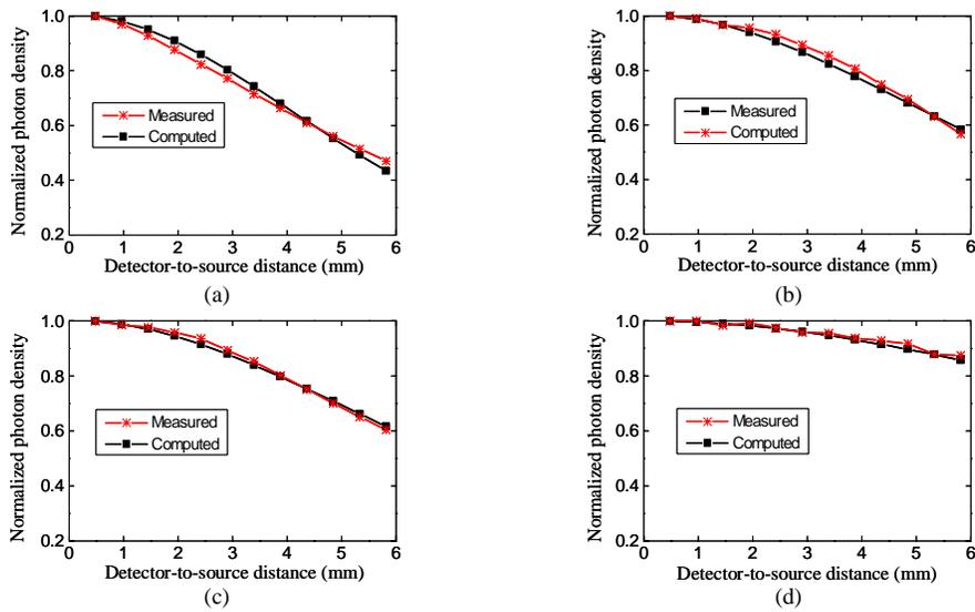
Fig. 11. Comparison of experimental and computational photon density profiles for determination of the optical parameters of the phantom materials: (a) Muscle (M), (b) Lung (L), (c) Heart (H), and (d) Bone (B).
