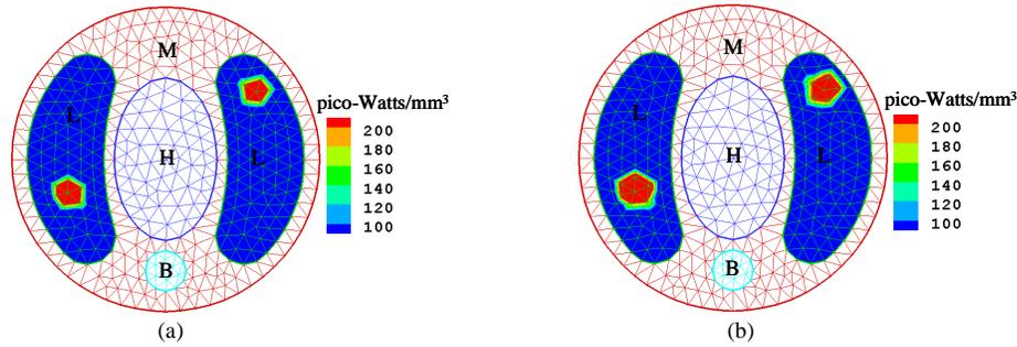
Fig. 2. Numerical simulation for BLT reconstruction of two sources in the left and right lungs, respectively. (a) The true source distribution with a density of 200.0 pW/mm<sup>3</sup> for each source, and (b) the counterparts reconstructed from the surface data corrupted by 10% Gaussian noise. The average density error is 3%.
