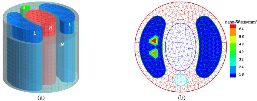
Fig. 13. (a) Finite element model for a middle portion of the mouse chest phantom. (b) Physical experiment on BLT reconstruction of two sources in the left lung of the mouse chest phantom. The difference between the reconstructed and real source centers was less than 1mm for both the sources at height 15.0mm. The maximum error of source power was about 18.5%.
