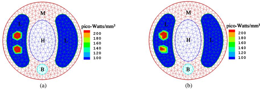
Fig. 3. Numerical simulation for BLT reconstruction of two sources in the left lung. (a) The true source distribution with density 200.0 pW/mm<sup>3</sup> for both the sources, and (b) the counterparts reconstructed from the surface data corrupted by 10% Gaussian noise. The average density error is 5%.
