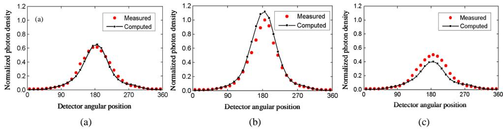
Fig. 14. Comparison between measured and computational photon density profiles along the detection circle on the phantom surface at heights (a) 10.6mm, (b) 15.9mm, and (c) 21.1mm, from the top surface of the model.
