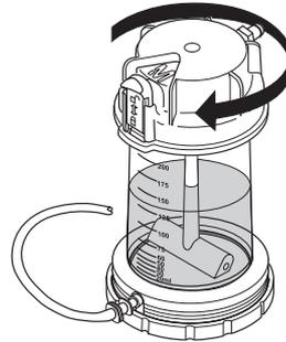
9. Move blue slide-lock downward to close pressure relief valve and lock cap in place.
