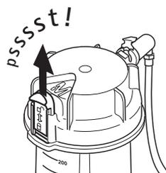
3. Disengage the quick-connect fitting by pressing down on the metal tab and pulling the fitting away from the cap.
