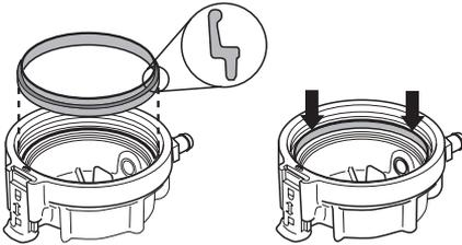
**IMPORTANT!** To avoid leakage between cap and cell body, make sure that the gasket is free of dirt/debris and oriented correctly in the cap.
