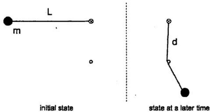
A ball of mass  $m$  is attached to a massless string of length  $L$ . The ball is released from rest as shown at left, with the acceleration of gravity  $g$  pointing down, and travels along a circular arc. As the ball reaches the bottom of the arc, the string starts wrapping around a nail (having a negligible diameter) located a distance  $d$  below the center of the arc.
