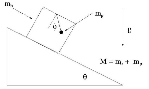
A hollow box of mass  $m_b$  sliding down an inclined plane has a pendulum of mass  $m_p$  attached by a massless, inextensible string as shown. Let  $\mu$  be the coefficient of kinetic friction between the inclined plane and the box.
