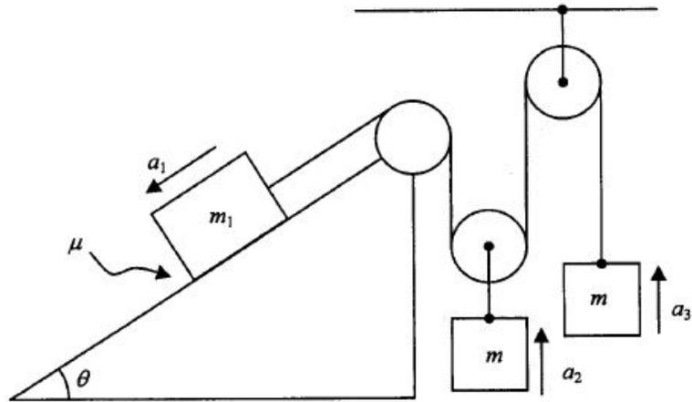
The following questions refer to the diagram above. All pulleys are assumed to be massless and frictionless and the inclined plane is fixed in place. The static and kinetic coefficients of friction between  $m_1$  and the plane are both  $\mu$ .
