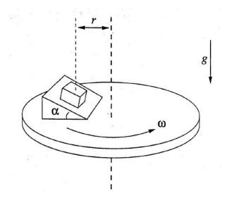
An inclined plane of angle  $\alpha$  is glued onto a horizontal turntable, as shown in the figure. A block is placed on the included plane a distance r from the axis of rotation of the turntable, and the coefficient of friction between the block and the plane is  $\mu$ . The turntable spins about its axis with constant angular frequency  $\omega$ .
