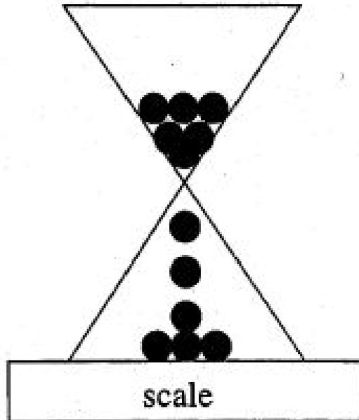
An hour glass of sand sits on a scale. Initially all the sand (of total mass  $m$ ) in the glass (of mass  $M$ ) is held in the upper reservoir. At  $t = 0$ , the sand is released and it falls at a constant rate  $dm/dt = \lambda$  to the bottom of the lower reservoir, as shown. Find the reading of the scale as a function of time.
