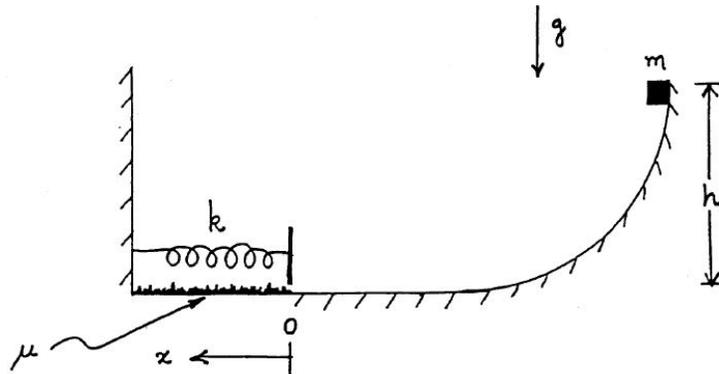
A block of mass  $m$  starts at rest and slides down a frictionless circular ramp from a height  $h$ . At the bottom, it hits a massless spring with spring constant  $k$  and in addition begins to experience a frictional force. The coefficient of kinetic friction is given by  $\mu$ .
