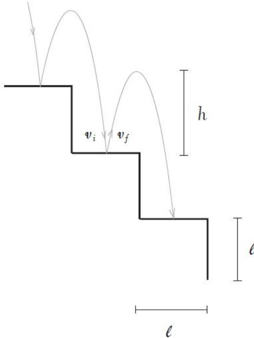
Each stair has the same height and depth  $\ell$ . The horizontal component of the marble's velocity is constant throughout, but the stairs have the property that  $-v_f/v_i = e$ , where  $v_i$  and  $v_f$  are the vertical velocity components just before and just after the bounce respectively, and  $e$  is a constant ( $0 < e < 1$ ).
