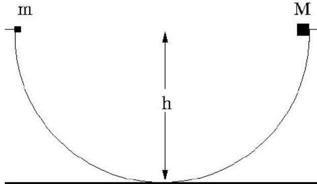
Two masses ( $M, m$ ) slide without friction (under the influence of a uniform gravitational field  $g$ ) down the sides of a hemispherical bowl. They each start with zero velocity at the lip of the bowl, which is a height  $h$  above the bottom.
