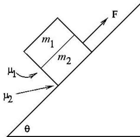
Upon an inclined plane of angle  $\theta$  is placed a block of mass  $m_2$ . Upon  $m_2$  is placed another block of mass  $m_1$ . The coefficient of static friction between  $m_2$  and the inclined plane is  $\mu_{2s}$  and the coefficient of sliding friction is  $\mu_{2k}$ . Likewise, the coefficient of static friction between  $m_1$  and  $m_2$  is  $\mu_{1s}$  and the coefficient of sliding friction is  $\mu_{1k}$ . A force  $F$  upward and parallel to the plane is applied to  $m_2$ .
