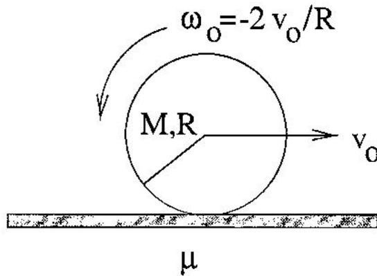
At  $t = 0$ , a solid sphere of mass  $M$  and radius  $R$  is spinning backwards while moving forwards on a table top of frictional coefficient  $\mu$ . The initial velocity of the sphere is  $v_0$  and the initial angular velocity is  $\omega_0 = -2v_0/R$  as shown below.
