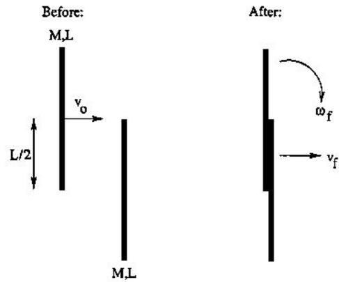
Two equal, uniform, thin rigid rods of length  $L$  and mass  $M$  collide and stick together, making a composite rod of length  $3L/2$ . Initially, one rod is at rest while the other approaches with speed  $v_0$  perpendicular to both rods.
