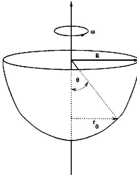
A small marble of mass  $M$  is placed on a hemispherical bowl of radius  $R$  as shown in the figure. If the bowl is spun (around its vertical axis) with the constant speed  $\omega$ , the marble eventually settles at a distance  $r_0$  from the axis.
