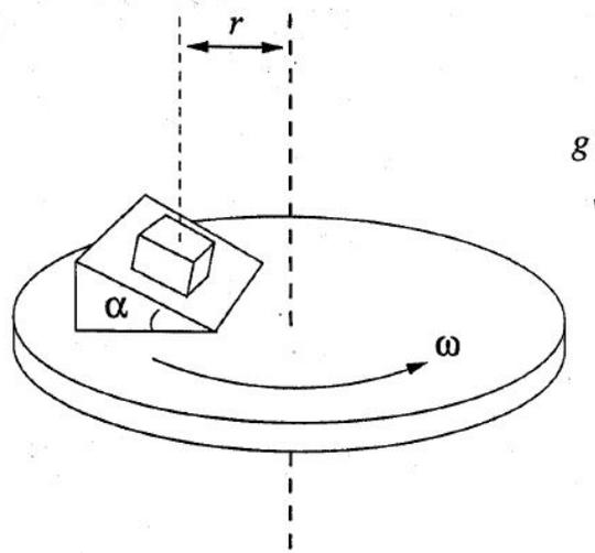
An inclined plane of angle  $\alpha$  is glued onto a horizontal turntable, as shown in the figure. A block is placed on the included plane a distance  $r$  from the axis of rotation of the turntable, and the coefficient of friction between the block and the plane is  $\mu$ . The turntable spins about its axis with constant angular frequency  $\omega$ .
