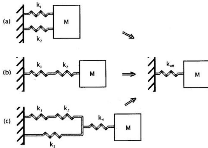
The restoring force on a spring is governed by Hooke's Law,  $F = -kx$ . Springs are linear devices, so any combination of springs can be modelled as a single spring with an effective spring constant  $F = -k_{\text{eff}}x$ . Refer to the diagram for parts (a), (b) and (c). Your final answer will not depend on  $M$ .
