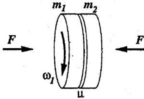
A rudimentary transmission can be made by forcing two uniform cylindrical wheels with frictional coefficient  $\mu$  together. The wheels have masses  $m_1$  and  $m_2$ , and both have radius  $R$ . Initially, wheel 1 is rotating with angular velocity  $\omega_1$  and wheel 2 is at rest. The wheels are being forced together with a constant force  $F$ , uniformly distributed across each wheel's face.
