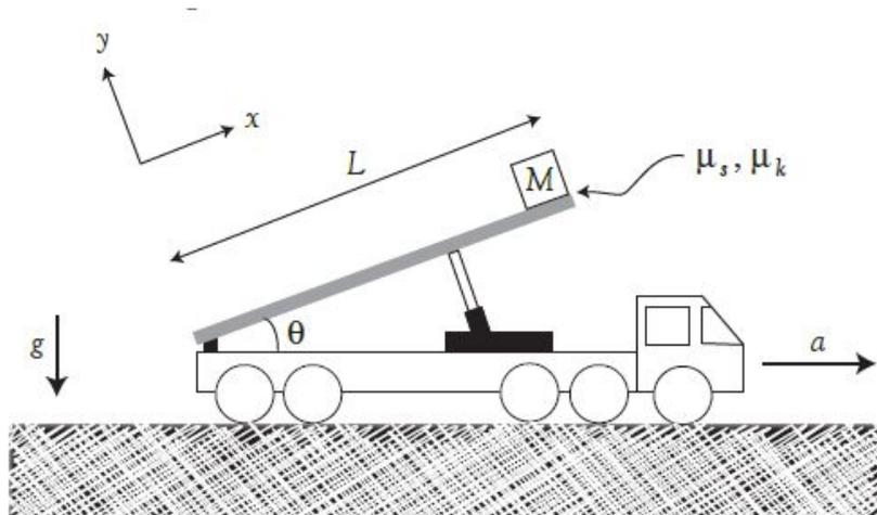
For this problem, use the  $x, y$  coordinate system shown in the figure. These coordinates are fixed with respect to the truck's bed, **not** to the ground.
